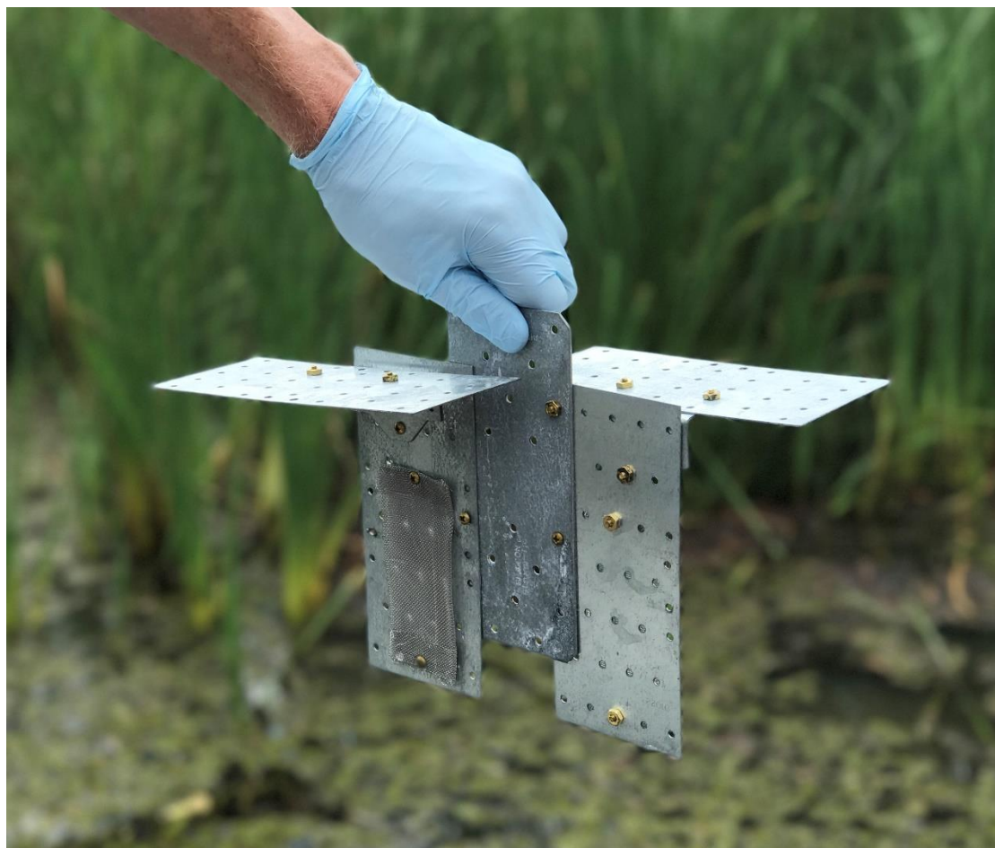
Figure 3. Passive sampler used at Lyons Creek East. PRC sampler is on the opposite side.
