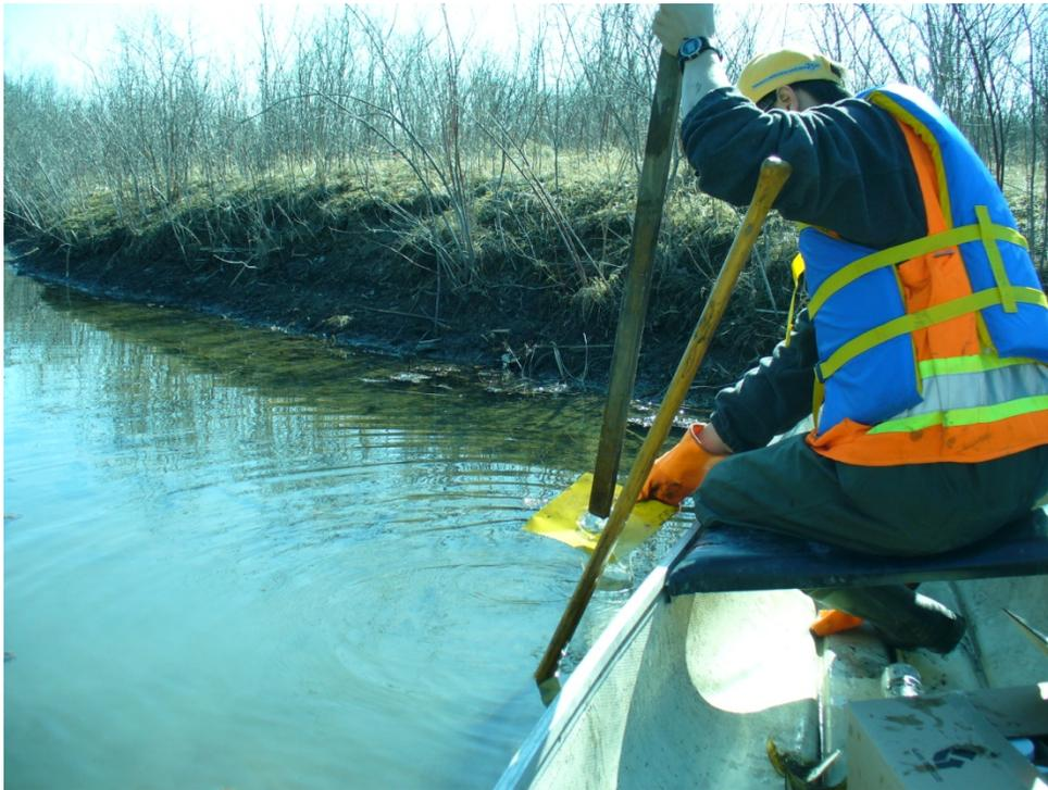
Photograph 7: Sediment traps being set
