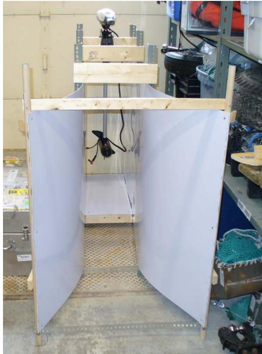
Photo 1: Flume with electric motor
