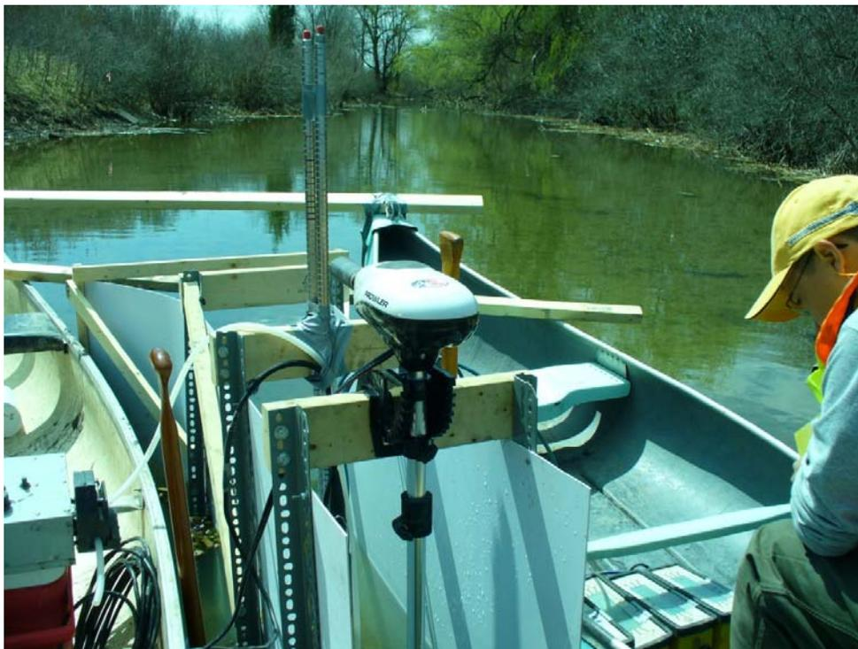
Photograph 4: Flume deployed in stream
