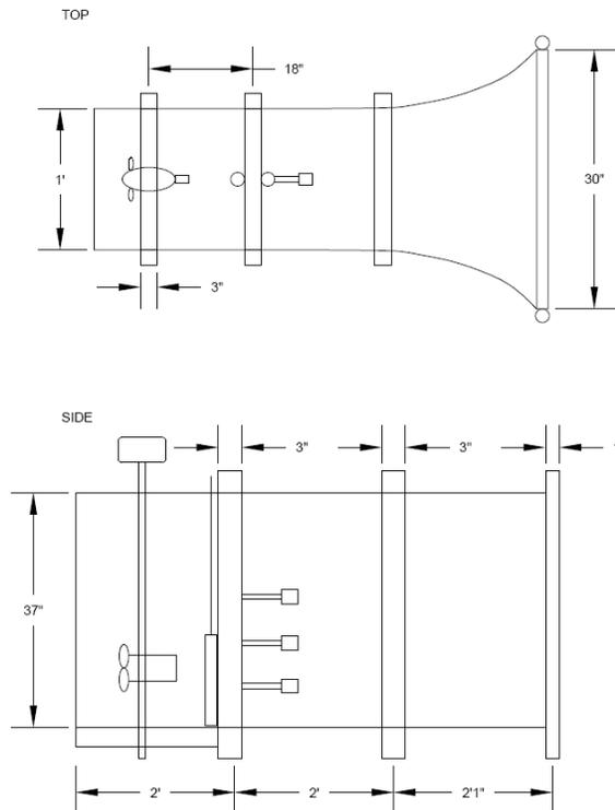
Figure 1: Flume Apparatus Diagram
