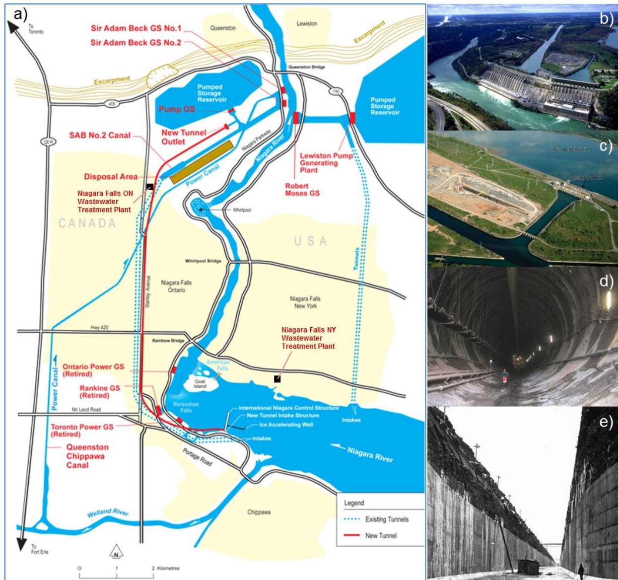
Figure 2. Map showing locations of hydroelectric power stations, water supply tunnels and wastewater treatment plants (a); and photographs of Sir Adam Beck Power Stations, canals and reservoir (b), detail of the pumped reservoir system (c), the new Niagara Tunnel completed 2013 (d) and the original Chippawa-Lewiston canal originating from the Welland River (e). Images are modified from Ontario Power Generation Niagara Tunnel Project portal ( http://www.opg.com/generating-power/hydro/projects/niagara-tunnel-project/ ).
